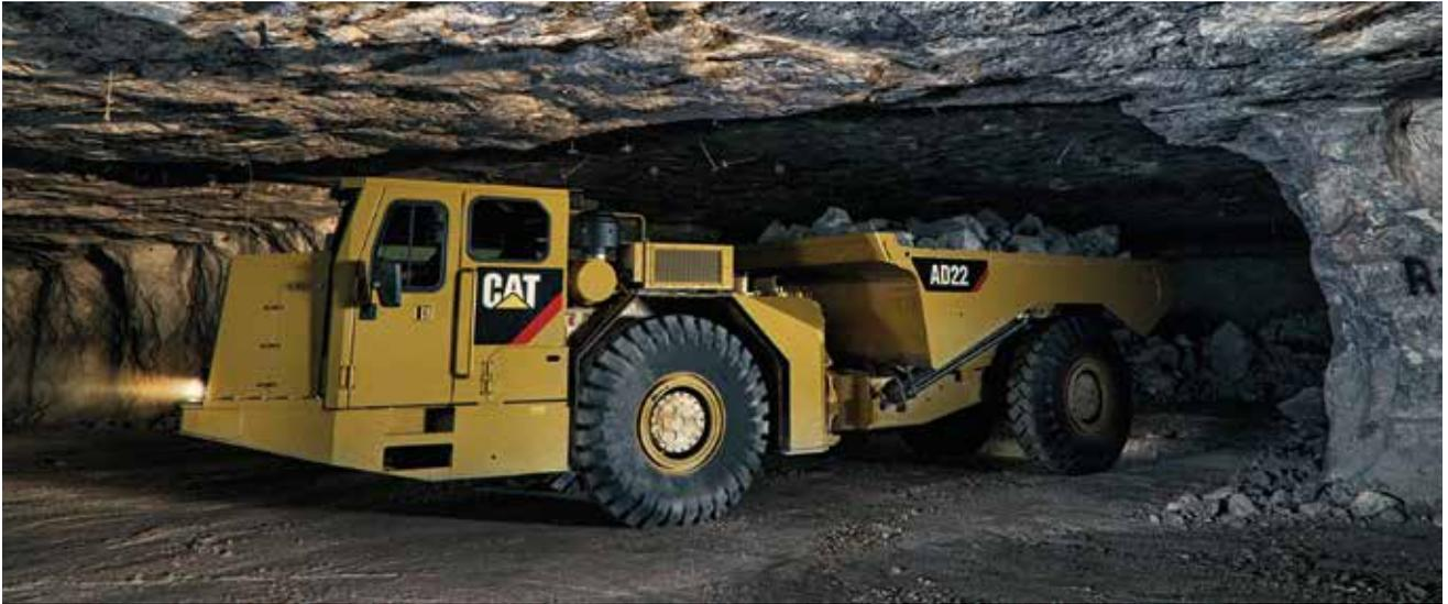
**The Cat AD22** ► the Cat underground truck line, the AD22, is Caterpillar's smallest but is designed to deliver the performance and durability of its larger counterparts. Its 22t payload is one of the largest in the size class.
