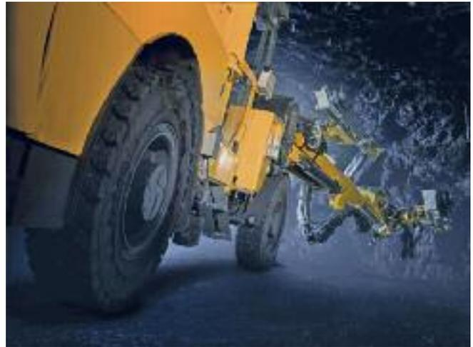
*Using an efficient and powerful electrical motor and battery drivetrain, Atlas Copco's Boomer M2C Battery is able to perform long tramping in challenging conditions without any emission at all*
