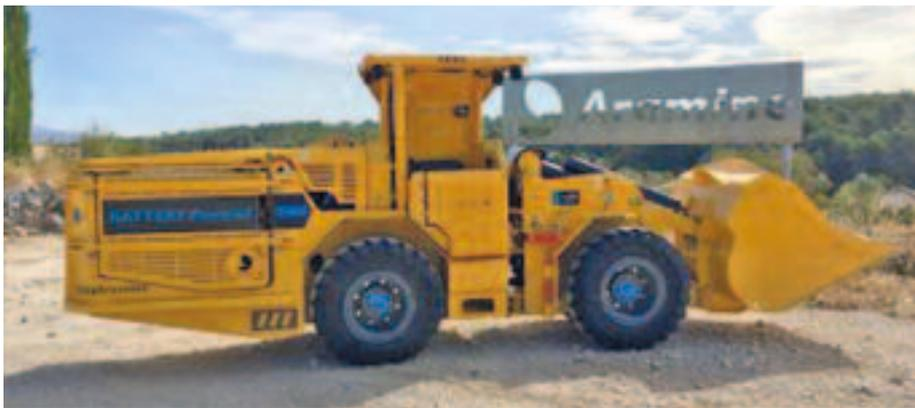
*The Aramine L140B has the same or even more breakout force than a diesel machine. The autonomy is approximately four hours depending on application and usage, which allows mucking three to four faces in one shift*
