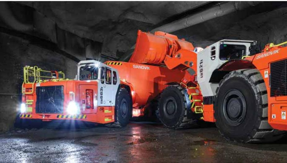
An LHD dumps its load in a new Sandvik TH663i truck.
