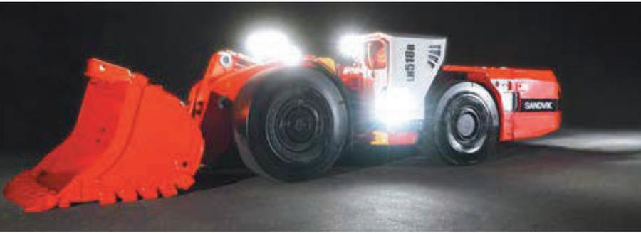
The new LH518B, Sandvik's first 18-t battery-electric loader. (Photo: Sandvik)
