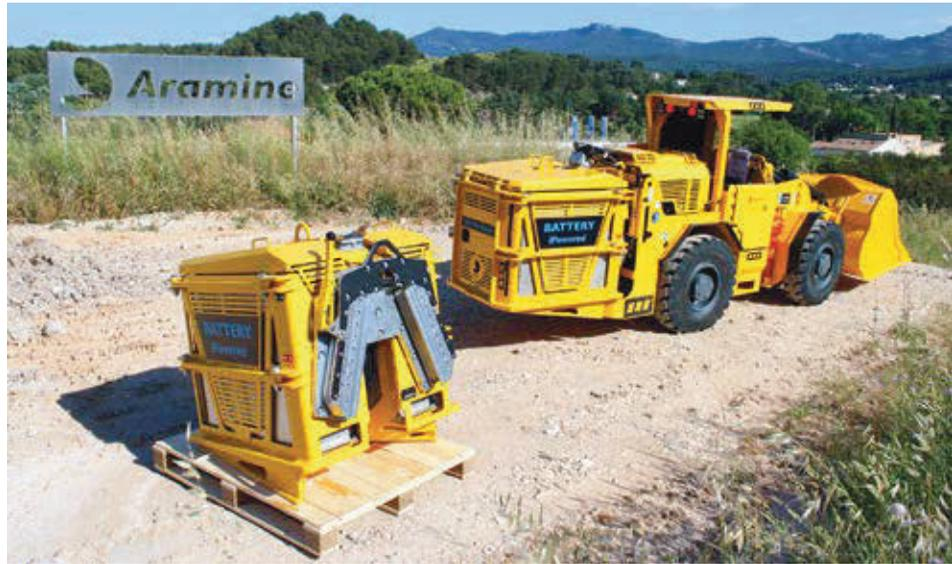
The miniLoader L140B QRS5 — the Quick Replacement System allows the battery to be changed out in less than 15 minutes. (Photo: Aramine)
