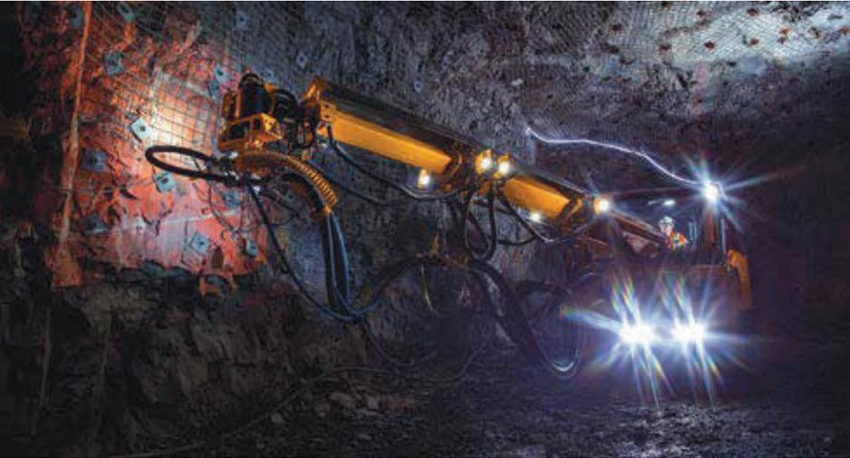
The new battery-powered SS5 shotcrete sprayer and TM3 tumbler are put through their paces at the MacLean test mine. (Photo: MacLean Engineering/Mining Industrial Photographer)
