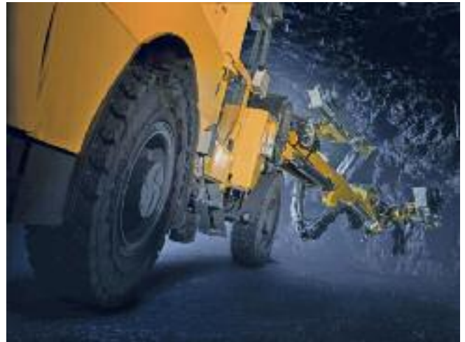
Using an efficient and powerful electrical motor and battery drivetrain, Atlas Copco's Boomer M2C Battery is able to perform long tramming in challenging conditions without any emission at all
