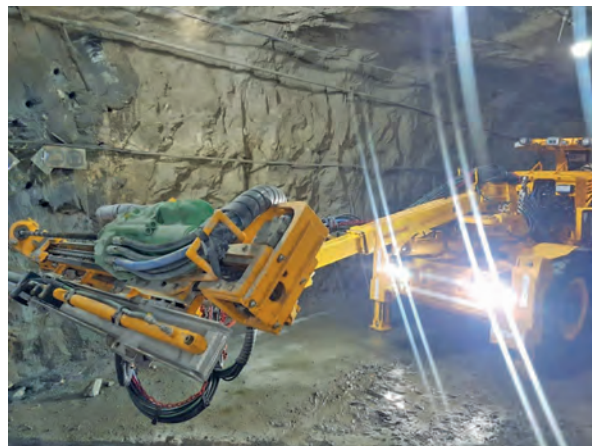
MacLean Engineering’s secondary breakers have been proving their worth in Africa, with a number of machines safely and effectively eliminating ore flow blockages and releasing trapped reserves above the draw point
