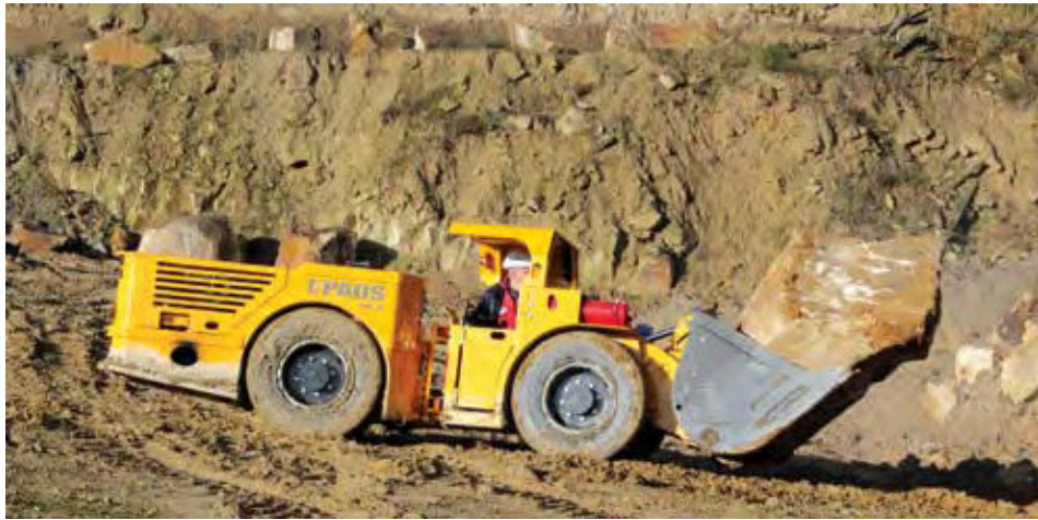
The PFL 8 LHD has a 0.8 m 3 bucket, a payload capacity of 1.5 mt, breakout force of up to 40 kN, an operating weight of 6.3 mt, and engine power of 69 kW. (Photo: Paus)
