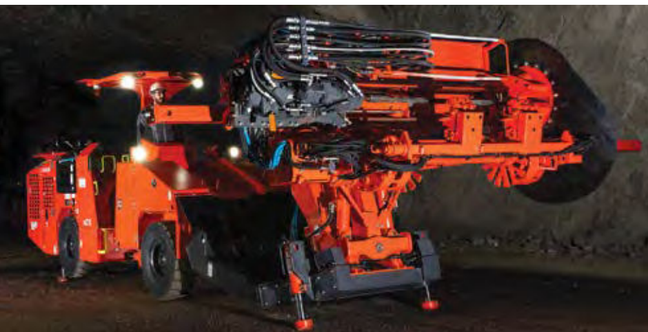
The DL2711 is a fully mechanized top-hammer longhole production rig capable of drilling vertical and inclined fans, single or parallel, 64- to 89-mm-diameter longholes, up to 38 m in length, using T38, T45 and T51 MF-rods or 65-mm tube rods. (Photo: Sandvik)
