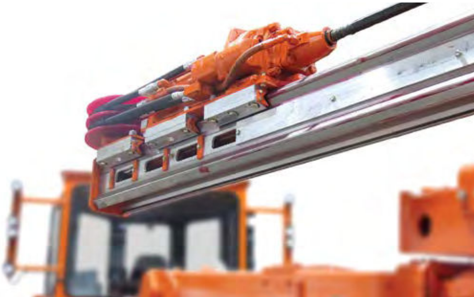
The HVL-38 offers an impact energy of 196 Nm, uses female striker bars, features a shorter feed length for reduced weight and improved mobility, and can be retrofitted on existing carriers. (Photo: J.H. Fletcher & Co.)
