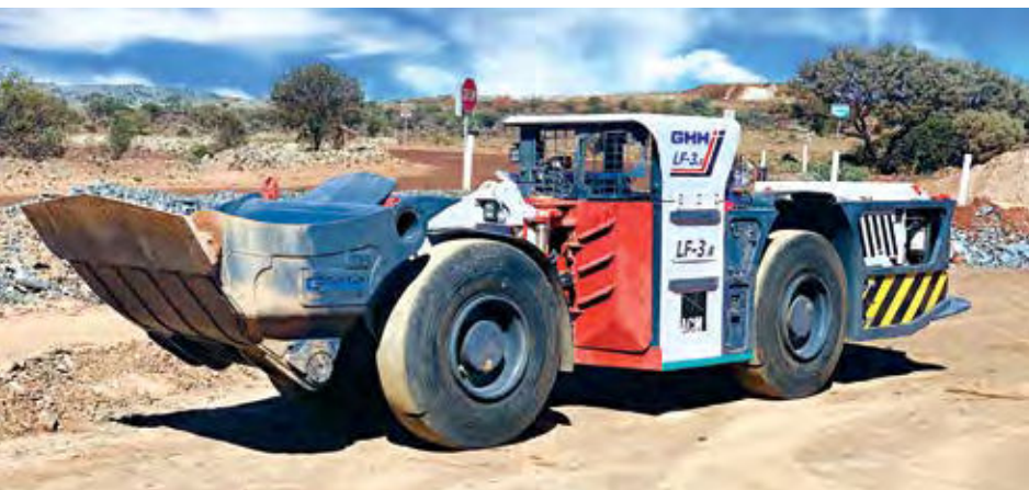
The LF-3 has an operating weight of 11 mt, a standard bucket capacity of 1.5 m 3 , and a payload capacity of 3.5 mt. (Photo: GHH)
