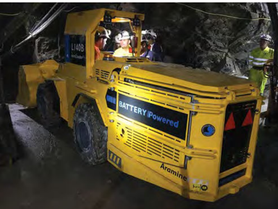
With a 0.7-m 3 bucket, the battery-powered L140B has a tramping capacity of 1,300 kg, tilt breakout force of 32 kN and lift breakout force of 35 kN. (Photo: Aramine)
