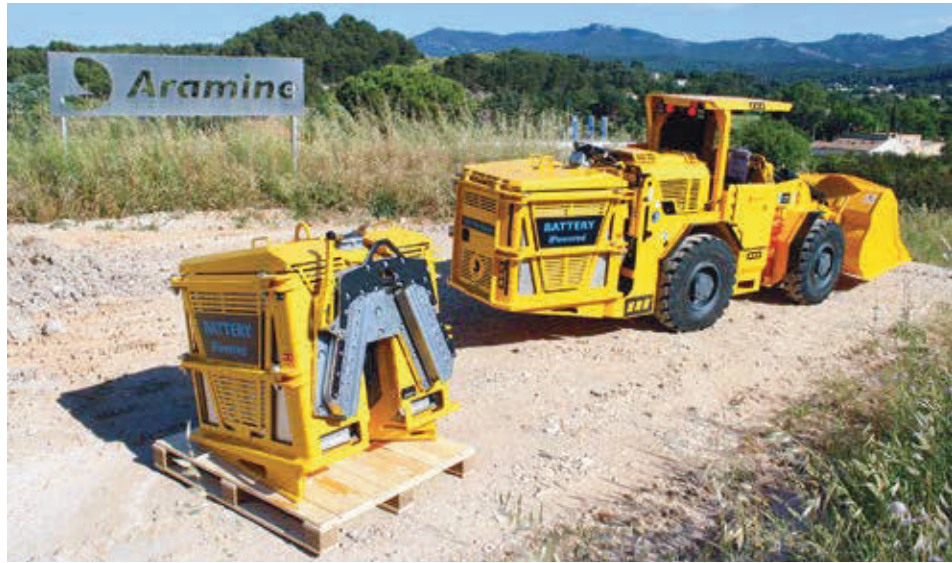
The miniLoader L140B QRS5 — the Quick Replacement System allows the battery to be changed out in less than 15 minutes. (Photo: Aramine)
