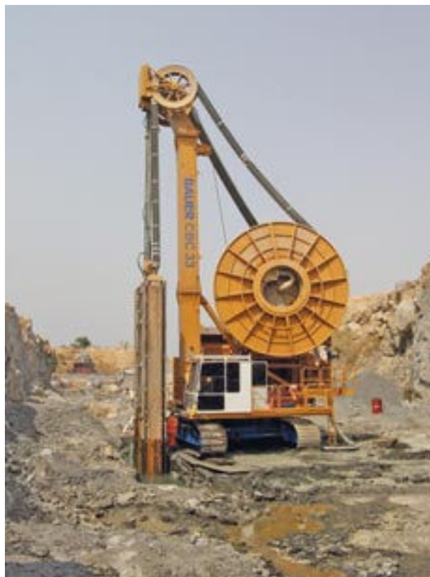
Looking to mine dykes for kimberlites to a greater depth, Koidu Limited and Bauer Technologies, in 2010, agreed to trial the BC 33 cutter at its kimberlite mining leases in Sierra Leone
