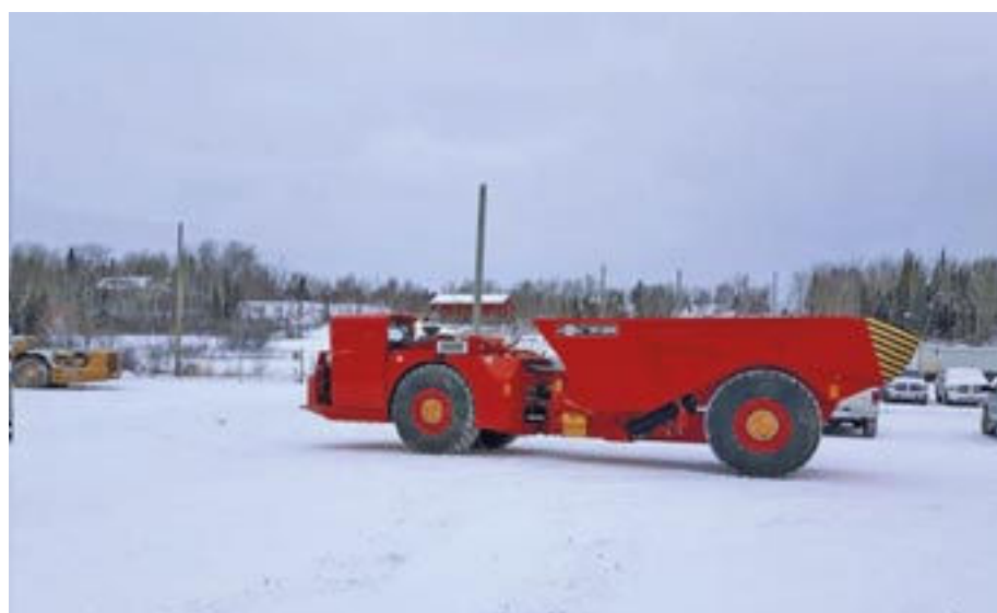
One of the more recent pieces of equipment to arrive at Pure Gold Mining’s Madsen gold project in Red Lake, Ontario, is a 26 t capacity DT-26N articulated dump truck from DUX Machinery. This underground four-wheel drive truck is well suited for hauling ore, waste and backfill on level and steep grades, according to DUX. It also has the highest power to weight ratio in its class, the company said, adding that it permits efficient chute, side and end loading in narrow drifts with low headings
