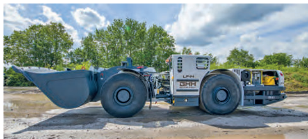
The GHH LF-14 is available with Tier 3, 4 and Stage V engine packages and has simplified, mine proven electrics that are IP 67 rated for exposed components
