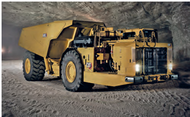
Caterpillar's new AD63 features a 5% increased payload and more torque for enhanced production capabilities, compared with its predecessor, the AD60
