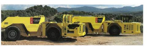
Aramine announced the final production runs of its T1601M, 15-ton mine trucks for small- to medium-scale underground operations. Deutz is discontinuing the F8L-413FW V8 air-cooled engines for the unit, which means final orders for the truck must be placed before end-of-year 2020.
