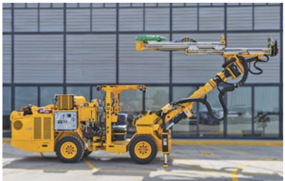
The MUKI FF is designed for tunneling development from 2 x 2 m up to 4 x 4 m
