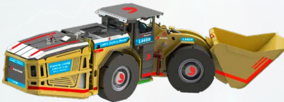
Figure 1. Aramine's L440B mining loader with a tramping capacity of 4.2 t, arriving in 2024.
