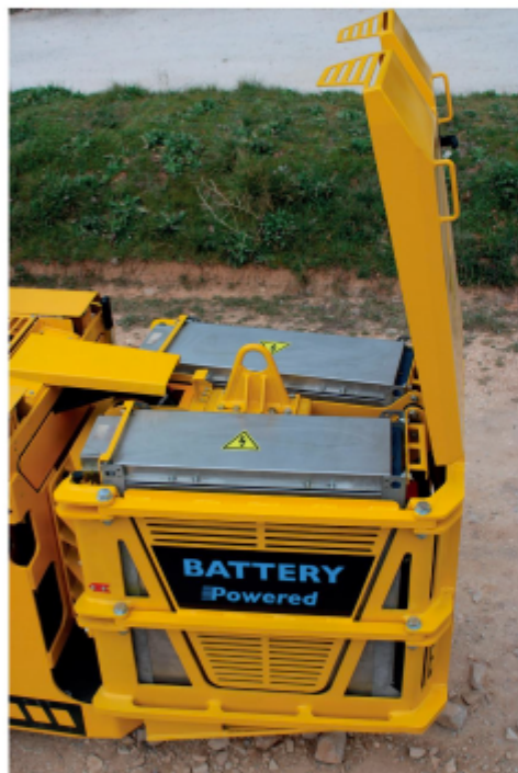
Figure 3. The battery energy module can be replaced in less than 5 minutes using a hoist.
