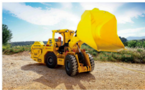
Figure 1. The L130E electric mining loader, with the cable reel at the back.
