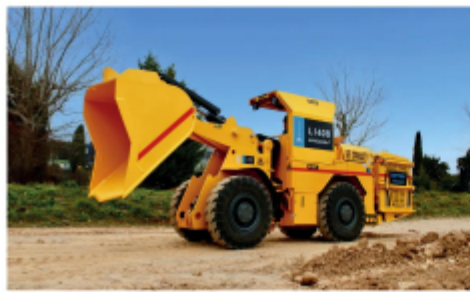
Figure 2. The L140B battery-powered mining loader, with a fully removable battery energy module.
