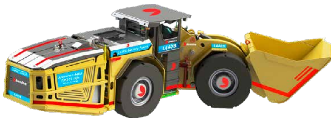
Figure 1. An L440B loader – the latest example of battery-powered mining equipment from Aramine.
