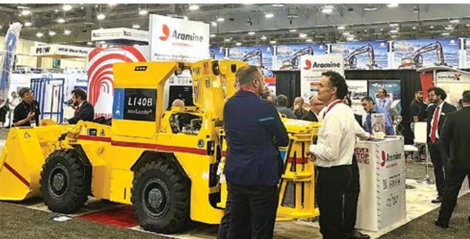
The rear segment of the above L440B loader is the detachable energy module, which can be replaced in 10 minutes, Aramine said at MINExpo. (Image: Aramine)
